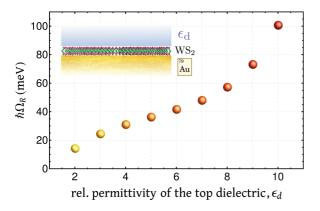
FIG. 3. Rabi splitting energy (in meV) as a function of the dielectric constant of the top insulator in dielectric/WS<sub>2</sub>/Au structures.
