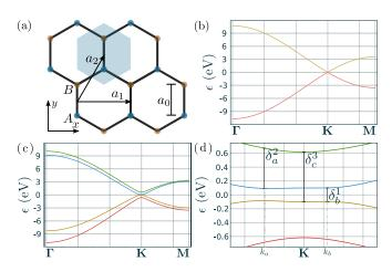
FIG. 1. (a) Representation of the monolayer lattice, including the primitive vectors and Wigner-Seitz cell (light blue hexagon). Energy dispersions for MLG (b), and BBG [(c) and (d)]. Plots (c) and (d) consider BBG with external bias potential  $\Delta = 200$  meV. In (d), we indicate some of the energy differences  $\delta_l^i$  occurring at the Van Hove singularities (VHSs) between the *i*th pair of bands, as listed in Table I.
