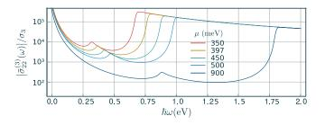
FIG. 4. Frequency dependence of the optical Kerr conductivity of MLG in units of  $\sigma_3$  for several chemical potentials  $\mu$ .
