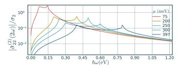
FIG. 5. SHG conductivities  $\bar{\sigma}_{22}^{(2)}(2\omega)$  of gapped graphene in units of  $\sigma_2 \equiv e^3 a_0/(4|\gamma_0|\hbar) = 2.88 \times 10^{-15} \text{ Sm/V}$  with  $E_g = \delta = 30 \text{ meV}$ .
