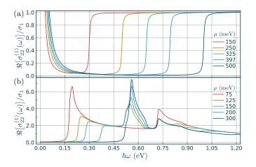
FIG. 2. Linear optical conductivity (in units of  $\sigma_1 = e^2/4\hbar$ ) for MLG (a) and BBG (b) as a function of energy for several  $\mu$  taking T = 1 K and  $\Delta = 200$  meV.
