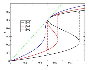
FIG. 3. (Color online) Bistability curves of the dimensionless field x as a function of y, for different values of the parameter  $\beta$ . When the power of the laser is increased the transmission through graphene follows the curve starting at zero until it reaches a point where the transmission suffers a sudden jump to higher values. The dashed-dotted straight line is the function x = y.
