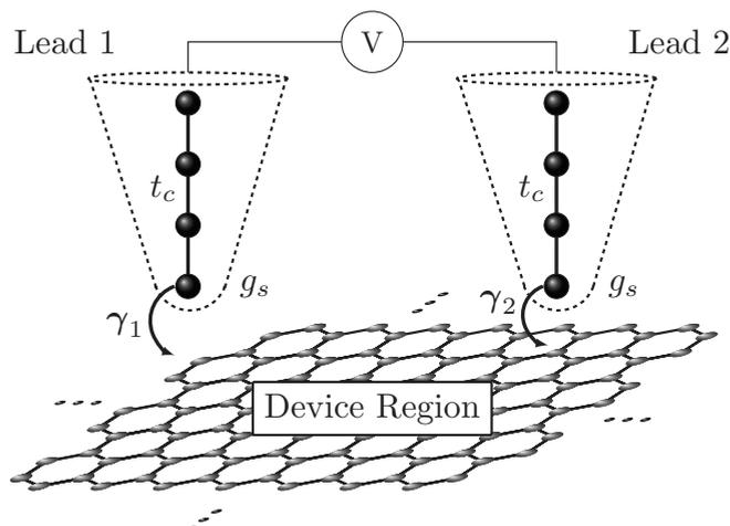
FIG. 1. Setup sketch including the leads modeled as one-dimensional chains with a hopping  $t_c$  between the sites. The surface Green's functions  $g_s$  are indicated together with the coupling  $\gamma^{1/2}$  between the lead and the graphene sample.
